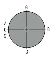
Supply connections A Barrier fluid IN B Barrier fluid OUT C Drainage G Grease S Flush
