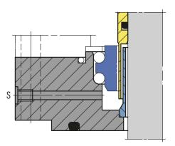
Can be used alternatively as wear trap with flush.
