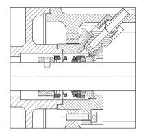
Mechanical seal with cooling of seal surface (connection with pump case)
